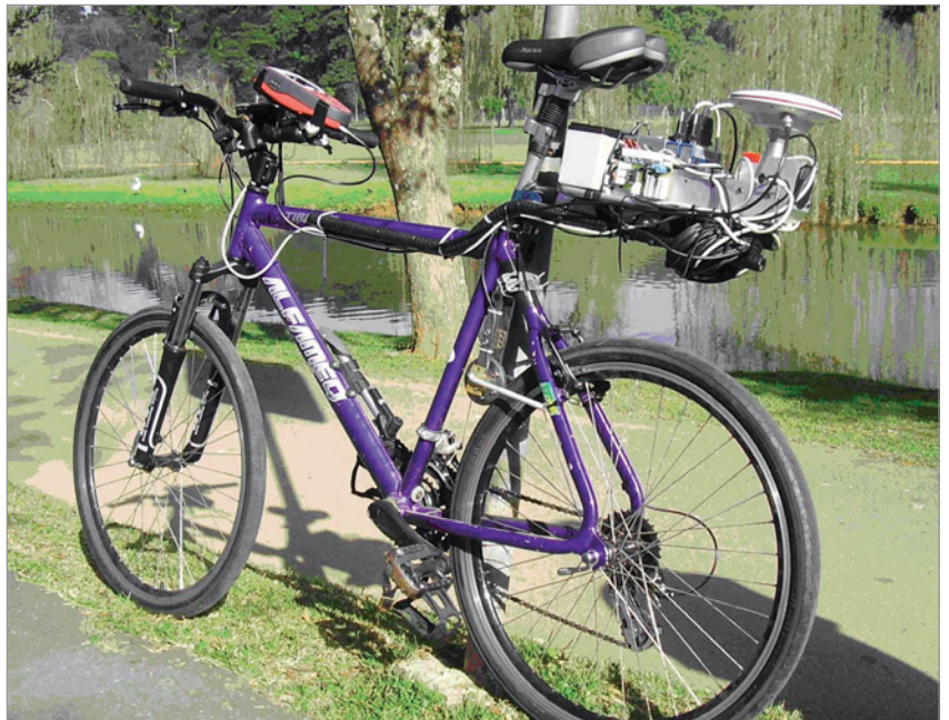
Figure 1: This first prototype of a pipeline inspection gauge (PIG) focused only on the high risk aspects of the geolocation algorithm. The bicycle was a creative way to move the electronic system at a rate comparable to the PIG.
