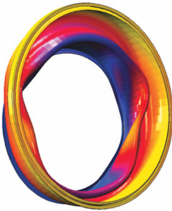
Nonlinear finite element analysis (FEA) of a coupler with MSC MD-Nastran including effects such as large deformation, buckling, and self-contact.
