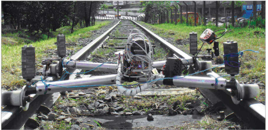
Figure 2: This second prototype of the EngeMOVI PIG reduced the degrees of freedom only to those that would be present in a pipeline by mounting the system on rails.
